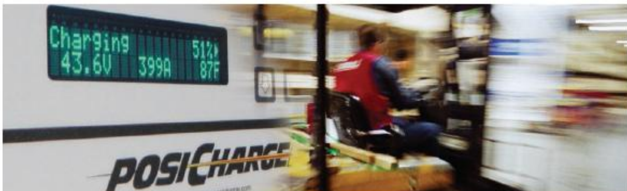
Fast charging can result in 75% less charging time compared to a standard lead acid battery charging system.
