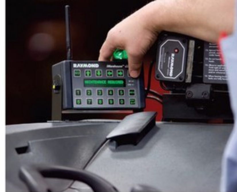
Truck-mounted hardware tracks data about whether a truck is idle or in motion, how much energy it uses, and can even produce collision reports including who, when and where.
