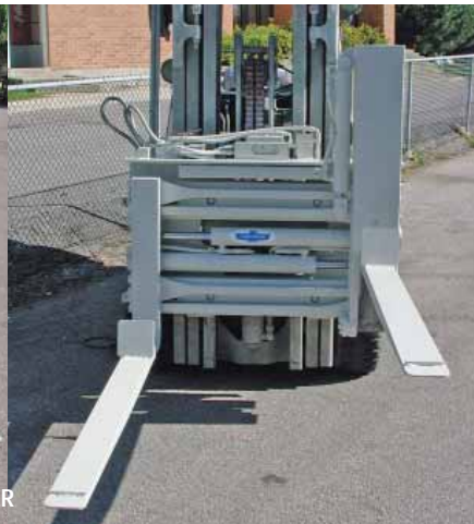
Frame Handler c/w Vertical Fork Adjustment Designed to handle Truck Frames
