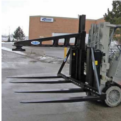
Frame Handler c/w Vertical Fork Adjustment Designed to handle Truck Frames
