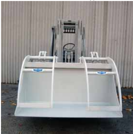
ITA Mounted Bucket with Grapple. Grapple Arms offer Load Securing feature
