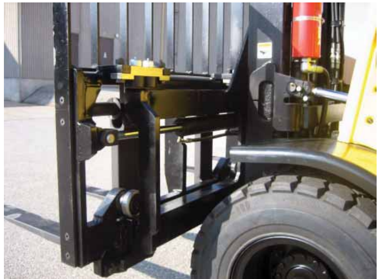
Double wide Block Handler with Roller design for easy maintenance.
