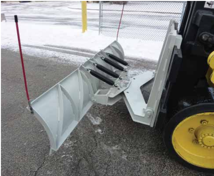
55C-SPC-63696 - Snow Plow Attachment. Also available as a Fork Pocket Mounting. Various widths & design
