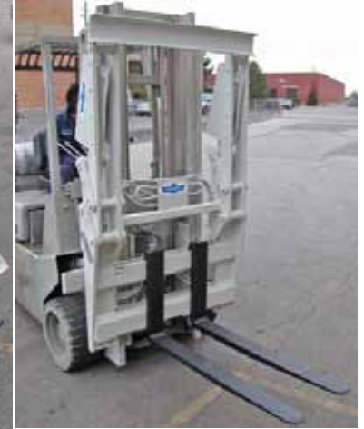
50C-BPV Broke Clamp with Vertical Opening Arm
