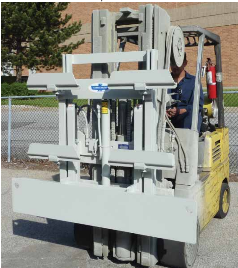
Special Lifting Blade Attachment for handling Appliances with "Folded Cap" packaging.
