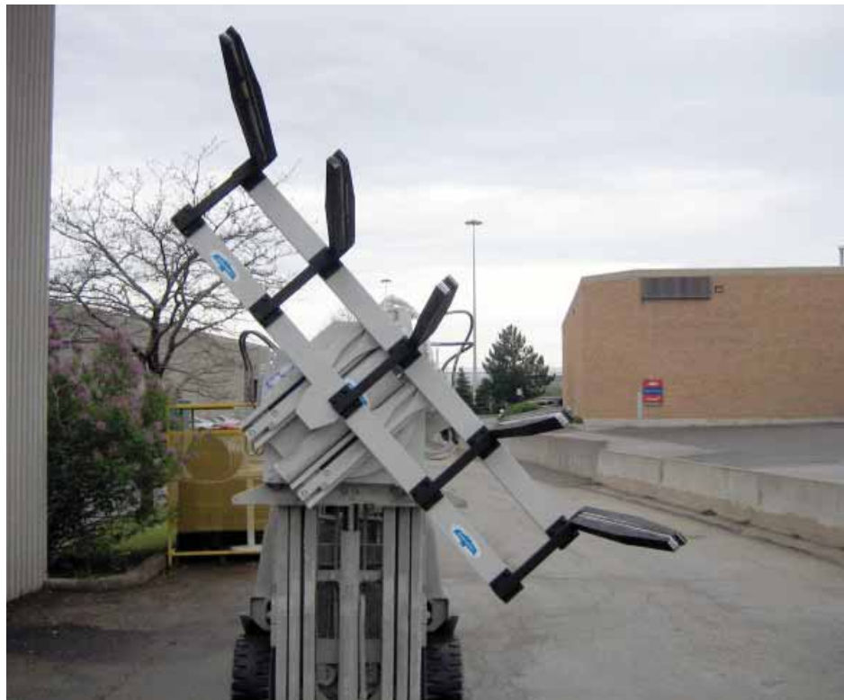
35D-TAL-62431 Designed for handling sheets of laminate ranging from 1/16" thick to 16" Thick
