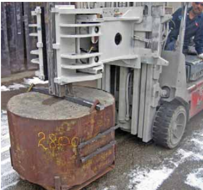
55C-AED-61981 Special Clamp Arm Frame to grab post of Anode
