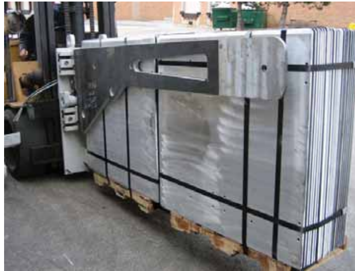
165D-MHB Special design to pick up complete load
