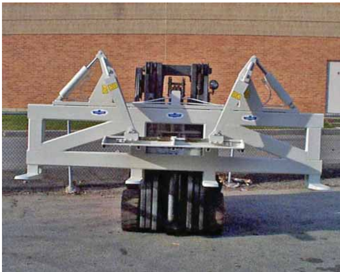
100C-FFS Special unit with Load Hold Down to handle stack of Steel Strips
