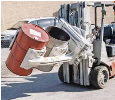
35D-DTR-SP to handle Two Drum Hinged Pads to Hand Various Diameters
