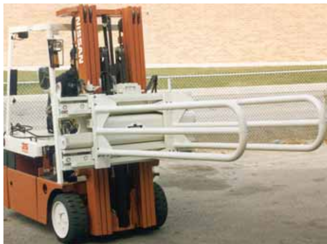
35D - With special tubular designed Arms to handle Foam
