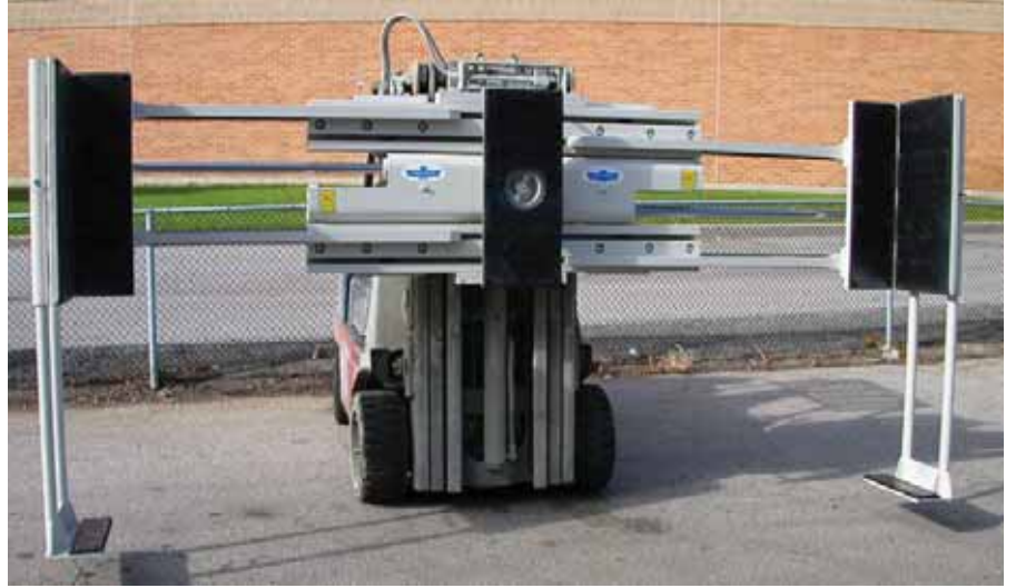
70D-MCR SP • Glass Handler Glass Adjustable Foot
