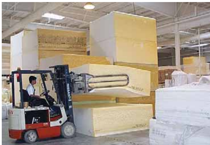
35D - With special tubular designed Arms to handle Foam
