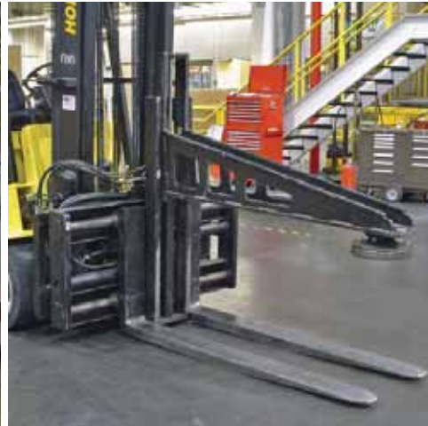
"C" Fork Positioner Hold Down Designed to handle stack of Steel plates
