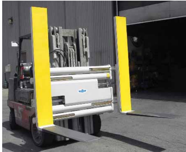
Fork Clamp with special Forks to handle Gypsum Slip on Poly Backs are required to protect Gypsum sheets
