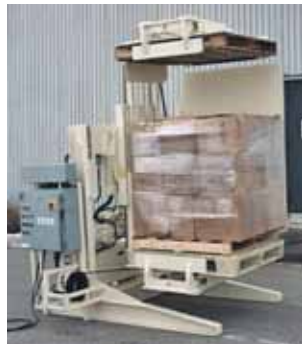
SLI Pallet Retention Pallet Retention Mechanism retains Top Pallet when load is inverted.
